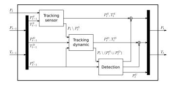
Fig. 2. Our framework consists of modules for motion detection, tracking the sensor, and tracking dynamic objects. Point sets are indicated with P, motions models with T.
