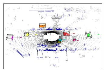
Fig. 1. A 3D LiDAR scan recorded by a car in a heavy traffic situation. Our approach estimates the motion of the car relative to the static structure, shown in blue, and the dynamic objects in its environment, shown in different colors. The arrows indicate the direction of the estimated motion.
