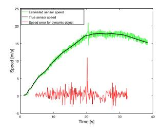
Fig. 5. Speed estimation for sequence A. The ground truth for the sensor motion is depicted in black, our estimate in green. The error in the speed estimation for the dynamic object is colored red.
