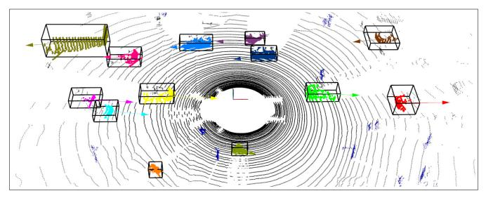
Fig. 3. LiDAR scan of sequence B at t = 26.2s. Ground truth is indicated by black bounding boxes. Structure classified as static is shown in blue, dynamic objects in other colors. Arrows display the translational part of the estimated motion models.
