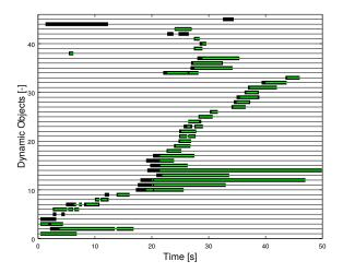
Fig. 4. Tracks for sequence B. Ground truth is depicted in black, estimated tracks are colored green. Gaps in the ground truth are caused by occlusions.
